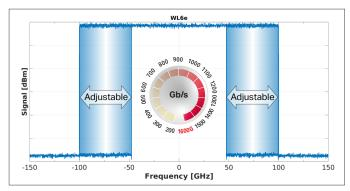
Granular Adjustable Line Rates, up to 1.6 Tb/s, which, together with Variable Baud (95–200 GBaud), allows for the optimal balance between capacity and spectrum based on client connectivity, network link characteristics, and channel spacing.
