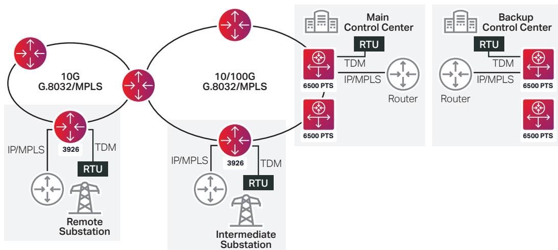
Figure 2. IO utility TDM network
